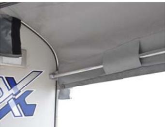
10. Insert side wall arms through sleeves on roof and the fit spigot end into holes on aluminium front beam and PVC rectangular cups against caravan side. Tension poles to suit.
