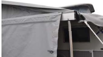
4. Introduce front wall bolt rope to extrusion on front of main aluminium beam.
