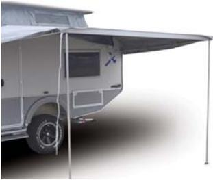
5. Lift front rail and open upright poles into vertical position and lock to desired height.
