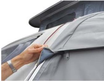
1. Introduce nose cone side wall bolt rope into tent extrusion.
