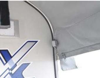
7. Zip closed corner gusset on both sides of tent and tension roof firmly.
