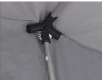
8. Lift up roof of patio in front and insert short centre upright pole into bracket on front aluminium beam. Ensure black 5 way fitting is fitted to top of pole so as not to damage roof fabric.
