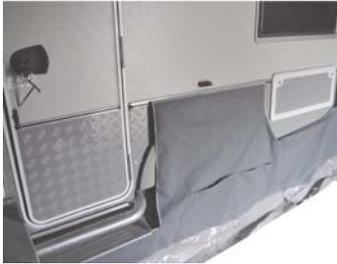
2. Thread bolt rope of draught skirt through extrusions on side and bottom of caravan.
